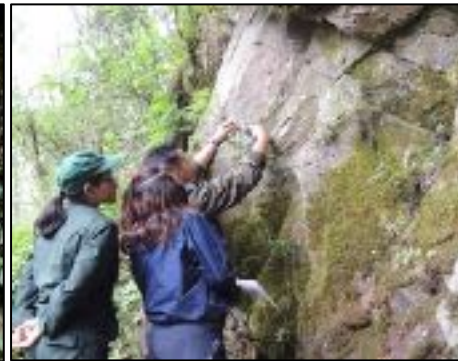
Figure 5: Measuring dip and strike of rocks
