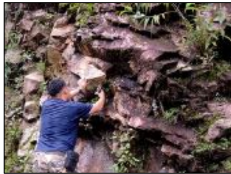
Figure 5: Measuring rocks with Brunton compass
