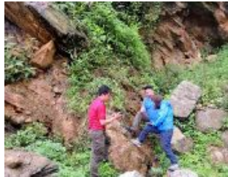
Figure 5: Measuring dip and strike of the rocks
