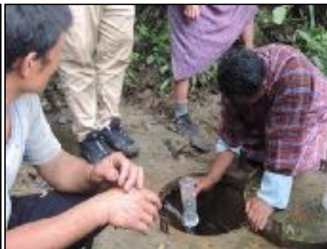
Figure 5: Measuring discharge of spring
