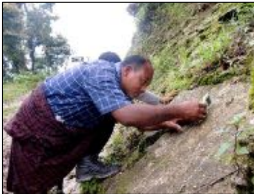
Figure 4: Measuring dip and strike of rocks
