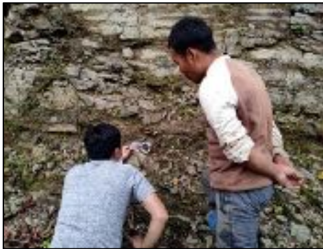
Figure 4: Measuring dip and strike of rocks
