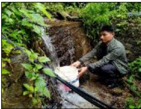
Figure 4: Measuring spring water discharge
